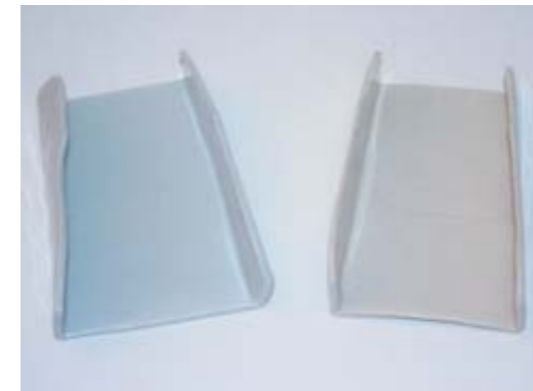
'Limoges' porcelain samples made by Anne Geroe Left-hand: Reduced; Right-hand: Oxidised. Translucency; Grey Straw
